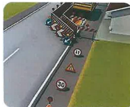
Figure 9 - Temporary construction site signs
