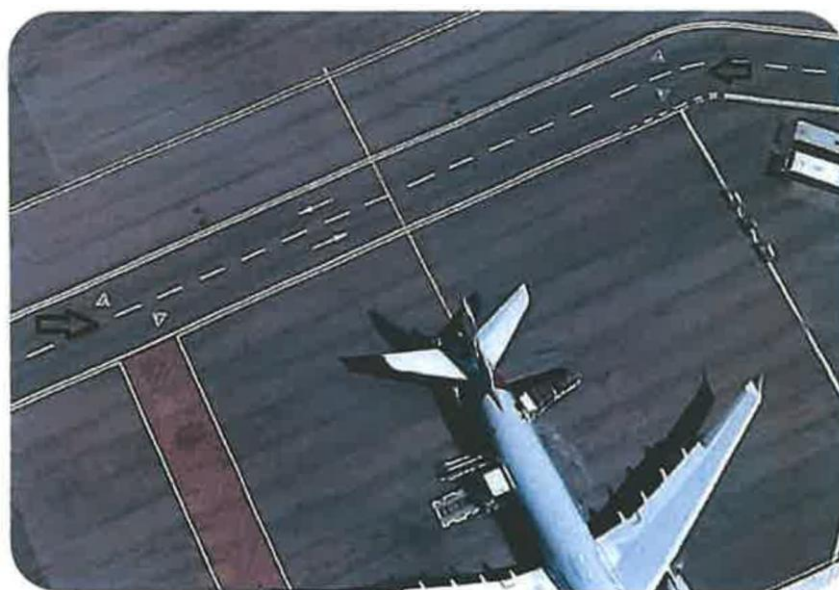
Figure 8 - Horizontal marking JET BLAST on the roadway
